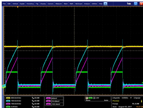
Figure 5: Over Power Protection Waveform
