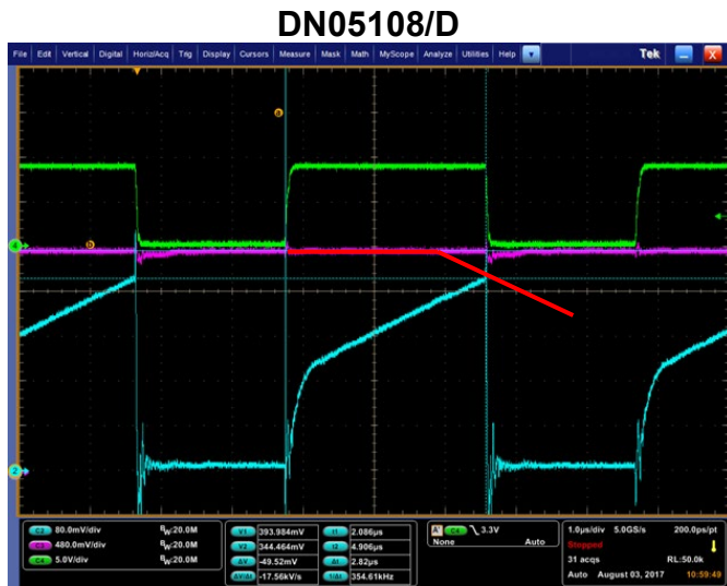
Figure 8: Slope Compensation Waveforms
